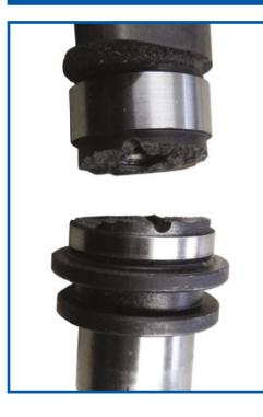
Appearance: Camshaft breakage between or through cam-lobes.
