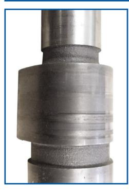
Appearance: Witness marking on base circle of cam-lobes, biased to one side. **Causes:** Worn hydraulic lifter and/or retainer springs. **Remedy:** Replace cam and followers if marks are deep, otherwise set tappets to correct clearance. Thoroughly flush the lubricating system and replace oil and filter.
