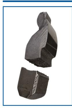
**Causes:** Mechanical overload resulting from:
